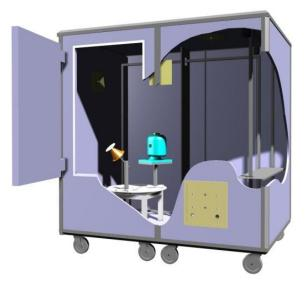
Figure 1. Drawing of the Bluetest HP700 reverberation chamber
