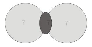
Figure 3: Two base-station setup with hand-over region. Note that cells are based on receiver power not on geometry.
