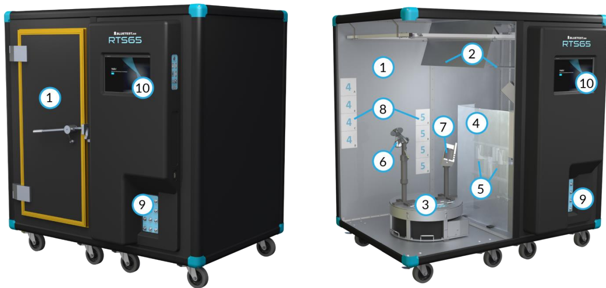
Figure 4, Bluetest RTS65 Reverberation Test System, exterior and interior
